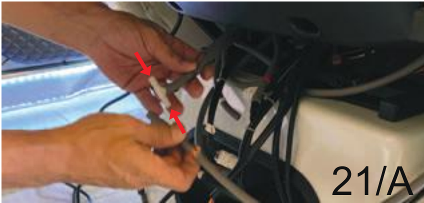
21/A Attach Brown Hose to Brown Hose (Left connection to "T" Hose)
