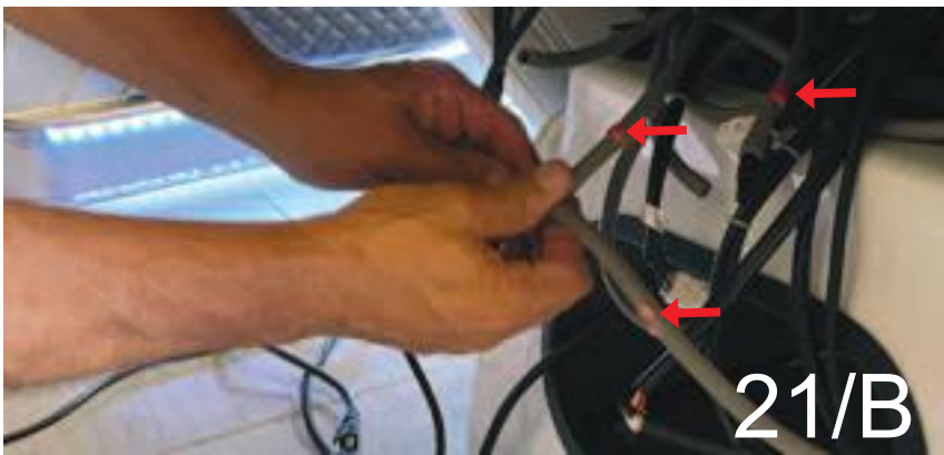
21/B Attach Brown Hose to Brown Hose (Right connection to "T" Hose)
